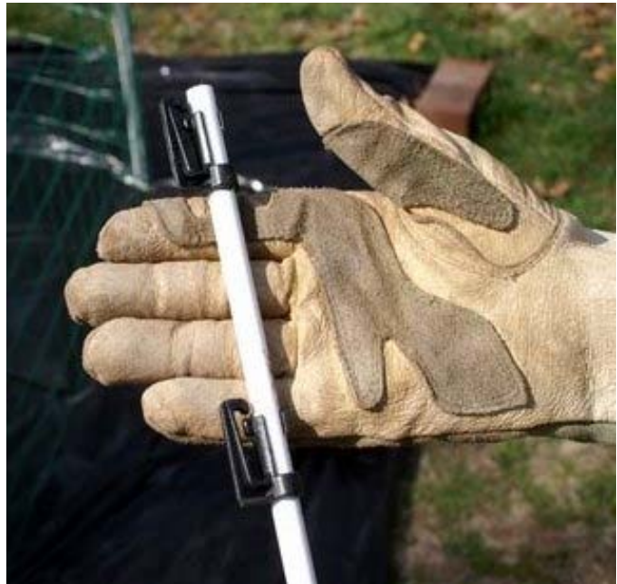
Step 6: Spacing the insulators 4" apart
